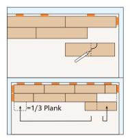
6. The width of the last row must be 1.5" or more (> 50 mm). To do this, place a full row of strips on top of the last row installed. Insert a 1/2" (12 mm) spacer against the wall, and using a full-width strip, trace a line the width of the final row from the wall. Cut strips for the final row to the designated width.
