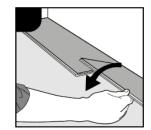
2. To engage the locking system, press the end of the board until you hear a click. A click indicates that the locking system is properly engaged.
