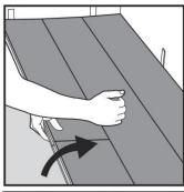
2. Disassemble the panels by sliding horizontally WITHOUT folding them.
