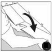
7. Angle the plank up and gently push forward until the plank locks into the plank of the previous row. Continue installing planks in the second row. After installing 2 or 3 rows, check for straightness using a string line, and adjust the first row if necessary due to unevenness in the starting wall.
