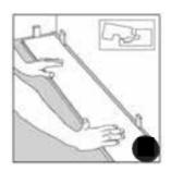
Assemble the end joints of the planks in the first row by inserting the tongue side into the groove side of the previous plank at a low angle. Gradually lower the plank down flat until the end joint closes, ensuring that the planks are perfectly aligned. Install remaining full planks in the first row.
