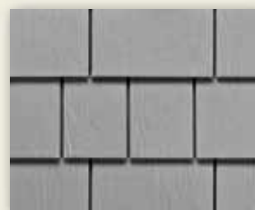
Individual Shakes Straight Edge 6-1/4" x 18" 8-1/4" x 18" 12" x 18" (8" exposure) Available primed only
