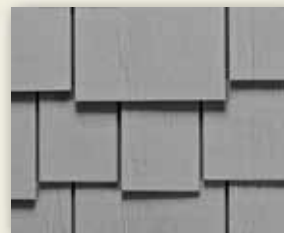
Individual Shakes Staggered Edge 6-1/4" x 18" 8-1/4" x 18" 12" x 18" (8" exposure) Available primed only
